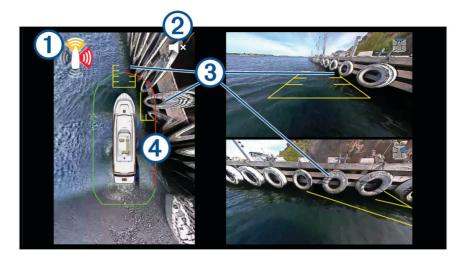
Proximity beeper alert notification. Indicates the area of the boat sending the proximity alert (port, starboard, bow, and stern). The color of the shaded area indicates the estimated severity of the alert:
